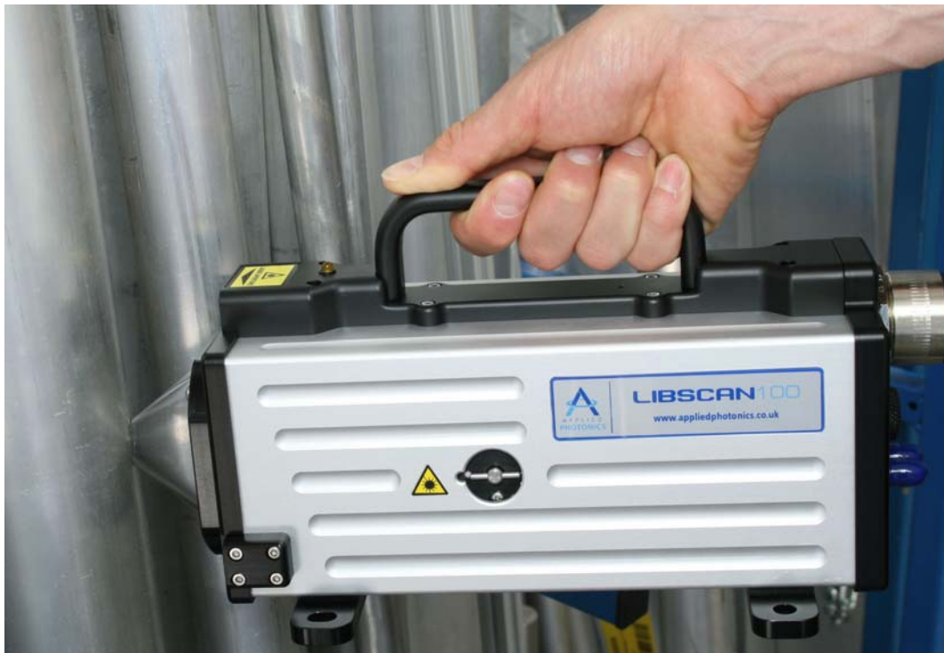
Free-style use of LIBSCAN for analysing large components ("open-beam", Class 4 laser product)
